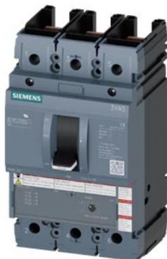
Автоматический выключатель 3VA5 UL Frame 250 3-pole, starter protection TM120M, AM, In=250A Without overload protection Short-circuit protection li=3...6 x In Without connection
