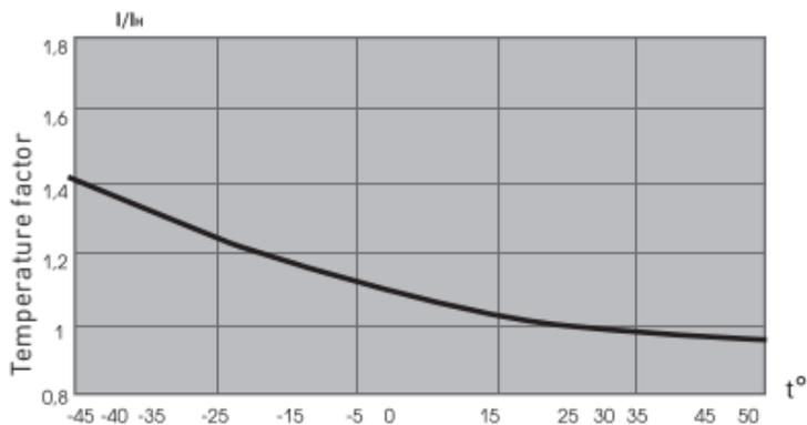
Figure 2. MCB temperature derating chart
