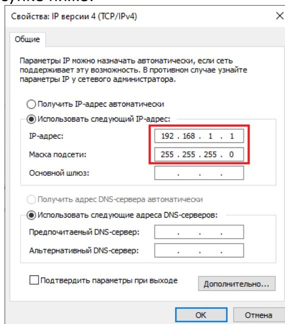
The screenshot shows the 'Свойства: IP версии 4 (TCP/IPv4)' dialog box. The 'Общие' tab is active. The 'Использовать следующий IP-адрес' option is selected. The IP address field is set to '192 . 168 . 1 . 1' and the subnet mask is '255 . 255 . 255 . 0'. Both fields are highlighted with a red rectangle. The 'Подтвердить параметры при выходе' checkbox is unchecked. The 'ОК' button is highlighted in blue.
