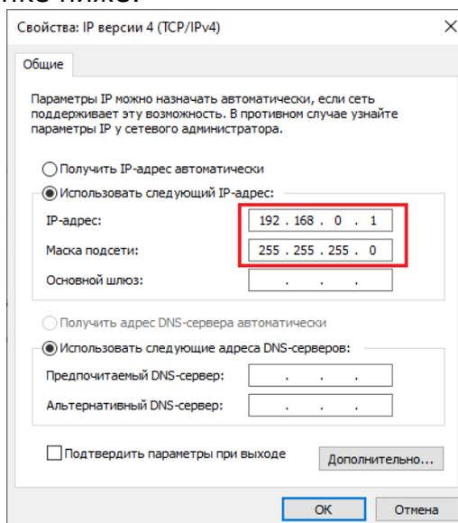
The screenshot shows the 'Свойства: IP версии 4 (TCP/IPv4)' dialog box. The 'Общие' tab is active. The 'Использовать следующий IP-адрес' option is selected. The IP address field is set to '192 . 168 . 0 . 1' and the subnet mask is '255 . 255 . 255 . 0'. Both fields are highlighted with a red rectangle. The 'Подтвердить параметры при выходе' checkbox is unchecked. The 'ОК' button is highlighted in blue.
