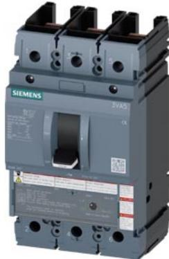
Автоматический выключатель 3VA5 UL Frame 250 Breaking capacity class C 100kA @ 480 V 3-pole, line protection TM210, FTFM, In=45A Overload protection Ir=40A fixed Short-circuit protection Ii=10 x In UL489 SB (naval), 50 deg. Cel Without connection
