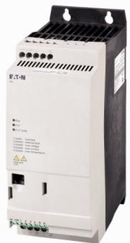
Variable speed starter, single-phase mains connection, three-phase motor connection at 230 V, 9.6 A and 2.2 kW / 0.3 HP
